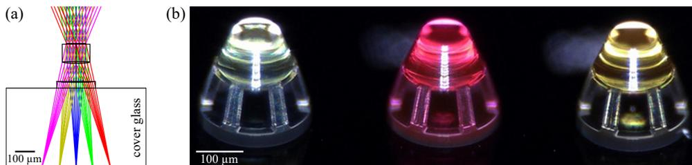
**Fig. 1.** Colored micro-optics. (a) Optical design of the lens system. (b) Microscope image of multiple micro-optics of different color printed successively on the same glass substrate.
