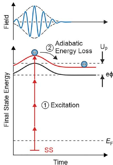
**Figure 3:** Energy-time diagram of the ponderomotive interaction in the adiabatic limit for 4th order electron emission. An electron is emitted at the maximum of the field envelope (step 1). As time progresses, the field envelope decays and the electron adiabatically loses the ponderomotive energy  $U_p$ , resulting in a down-shift of the electron's final-state energy (step 2).
