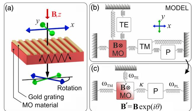
FIG. 1. (a) Schematic drawing of the hybrid magnetoplasmonic nanostructure. (b) Mechanical analog that represents the coupling of the relevant optical excitations. (c) Simplified oscillator model providing analytical solutions.
