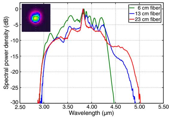
**Fig. 3.** Spectral broadening of the supercontinuum at maximum output power of 550 mW as a function of fiber length for a pump wavelength of 3.83  $\mu\text{m}$  and a core diameter of 9  $\mu\text{m}$ . (Inset) Mode profile for the 23-cm fiber at maximum output power of 550 mW.
