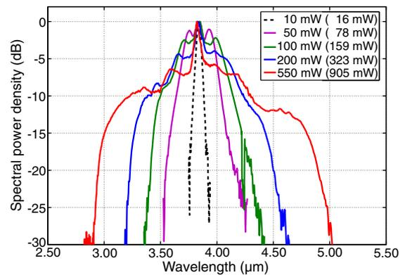
**Fig. 4.** Spectral evolution of the supercontinuum as a function of measured output power (input power) for a wavelength of 3.83  $\mu\text{m}$  and a fiber length of 23 cm and a core diameter of 9  $\mu\text{m}$ . SPM as broadening mechanism in the normal dispersion regime is visible as symmetric spectral evolution.
