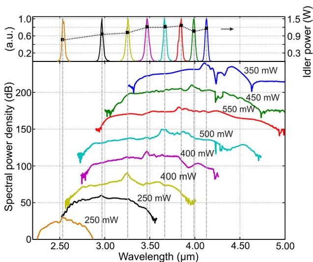
**Fig. 2.** Spectral broadening of the supercontinuum at maximum output power as a function of the launched idler wavelength for a fiber length of 13 cm and a core diameter of 9  $\mu\text{m}$ . For better visibility, each spectrum is shifted upward by 30 dB. The average output power correspond to pulse energies between 6 and 13 nJ.
