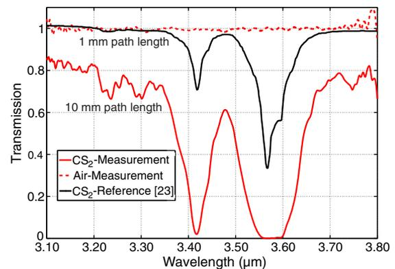
**Fig. 5.** IR-transmission spectrum of liquid carbon disulfide ( $\text{CS}_2$ ) measured with the supercontinuum source at a pump wavelength of 3.47  $\mu\text{m}$  and 100 mW output power. For comparison, we also plotted an air reference measurement and the reference data from NIST [23].
