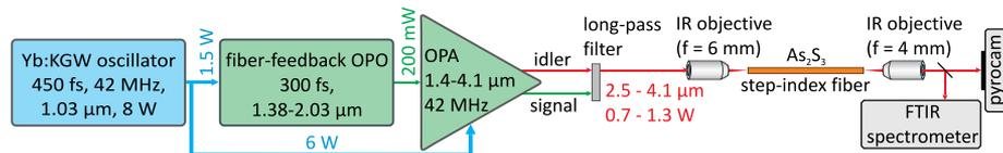
**Fig. 1.** Schematic of the experimental setup consisting of the laser amplifier system, step-index chalcogenide fiber, Pyro-camera, and FTIR-spectrometer.
