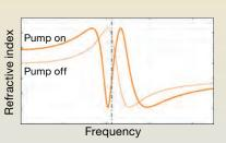
(Left) A characteristic probe absorption spectrum of an atomic medium under EIT conditions. The broad absorption peak experienced by the probe beam is split in two by a narrow dip when the pump is applied. (Right) This results in a very sharp variation of the refractive index, which is responsible for long pulse delays and slow-light behavior.
