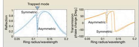
(Left) Suppression of scattering in the asymmetrically split-ring metamaterial leads to a narrow minimum of reflection losses, splitting the symmetric ring reflection peak in two. (Right) At the same time, the phase change of the transmitted wave exhibits steep normal dispersion, leading to low group velocities and long pulse delays.
