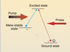
Typical three-level atomic system used in demonstrations of EIT.
