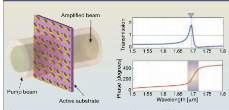
Loss-compensated slow-light device: metamaterial array with EIT-like dispersion placed on a gain substrate ( $\epsilon$ =9.5+035i). At the wavelength of 1.7  $\mu$ m, it shows single-pass amplification and simultaneously sharp normal dispersion.
